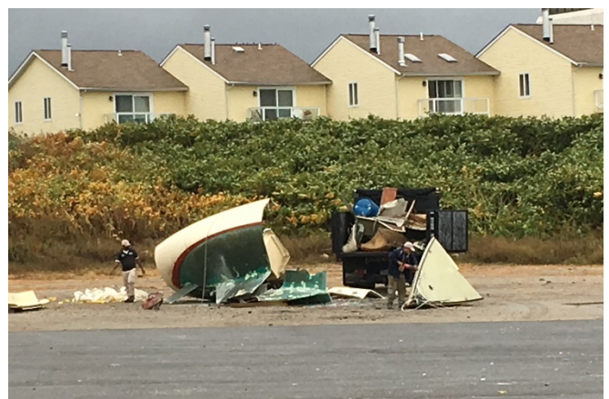
Figure 4. The yacht had to be cut into sections small enough to be taken for recycling
